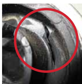
TORN BUSHING Load forces will tear bushing from sleeve
