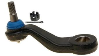
**STEERING IDLER ARMS** serve as a pivot point for the steering linkage assembly in your vehicle. The steering idler arm is attached on the opposite side of the center link from the Pitman arm and to the vehicle frame, which supports the center link.
